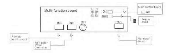
Note: It must use shield cables to connect with Non-poplar wired controller. The length should not exceed 50m.
