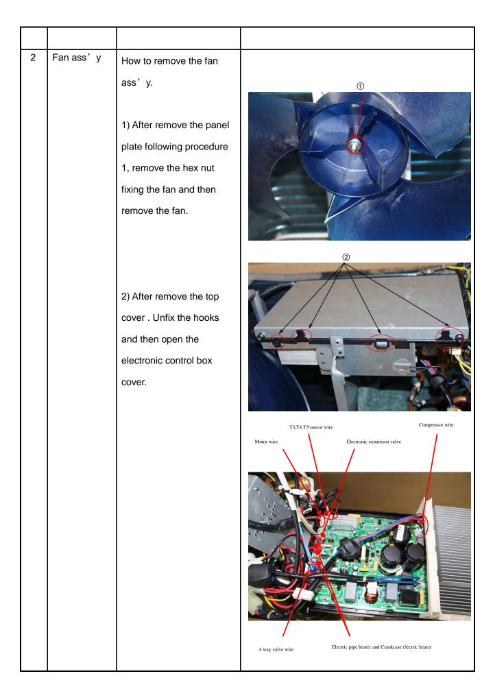
3) Disconnect the 3 connector for fan motor from the electronic control board. 4) Remove the four 4 fixing screws of the fan motor. Then remove the fan motor. 3 Electrical How to remove the parts electrical parts. 1) After finish work of item 1 and item 2, remove the connectors for the compressor and reactor.
