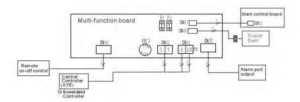
Note: It must use shield cables to connect with 4-cored wired controller and Central controller. The length should not exceed 50m.
