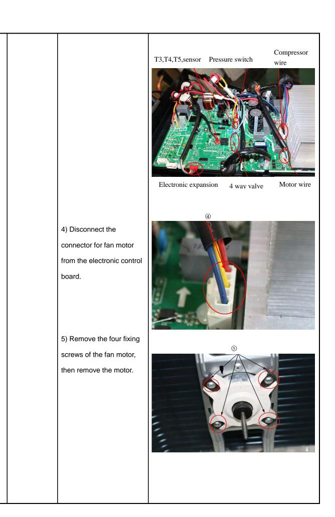
3 Electrical How to remove the 1 parts electrical parts. 1) After finish work of item 1 and item 2, remove the connector for the compressor 2 2) Pull out the two blue wires connected with the four way valve. 3) Pull out connectors of the, condenser coil temp. sensor(T3),outdoor ambient temp. sensor(T4) and discharge temp. sensor(T5).
