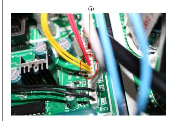
5) Disconnect the electronic expansion valve wire from the control board
